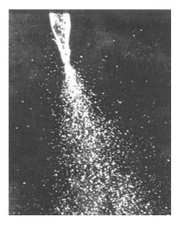
**FIGURE 1.2** Manipulate infectious fluids carefully to avoid spills and the production of aerosols and droplets. This photomicrograph shows the copious production of aerosols and droplets when the last drop in a pipette is blown out. Enough material can be aerosolized by such practices to create an infectious dose of some agents. Courtesy, National Institutes of Health.
